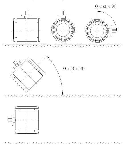
Valves with stem extensions (high end extensions) must be installed with vertical stem only. Please note that stem extensions must not be exposed to bending forces or torques.
