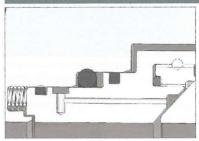
Both seals in the valves with the "Double Piston Effect" (DPE) actively participate in the internal sealing of the valve. In the case of any damage to one of the seals, the tightness of the valve is ensured by a second seal thanks to their special construction.
