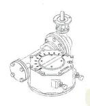
Worm Gear can be provided with Motor actuator Input flanges to accept standard ISO Mounting Base
