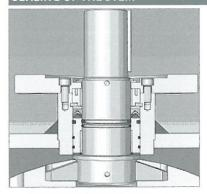
The sealing of the stems used in the valves manufactured by BROEN depends on the operating temperatures of the valve and the working medium for which the given valve is dedicated.
