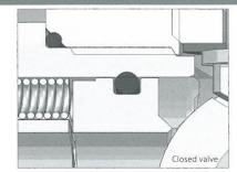
The tightness of the valve is ensured by the seals made from PTFE, PTFE + C or POM materials.
